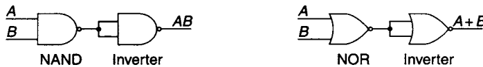
Figure 2.21 Complete sets formed by (a) series combination of two NAND gates and (b) series combination of two NOR gates
